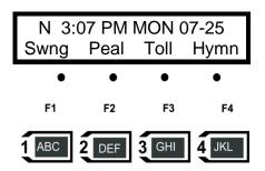
This is **Standby mode** displaying the season, time, day and date. The bottom line holds the labels for the **function buttons** which are the top four alphanumeric buttons.
