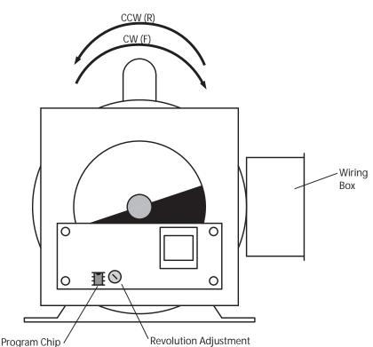
Clockwise Wiring 240V: Black, White and Orange from the motor housing are tied together. Red and Yellow are hot.
