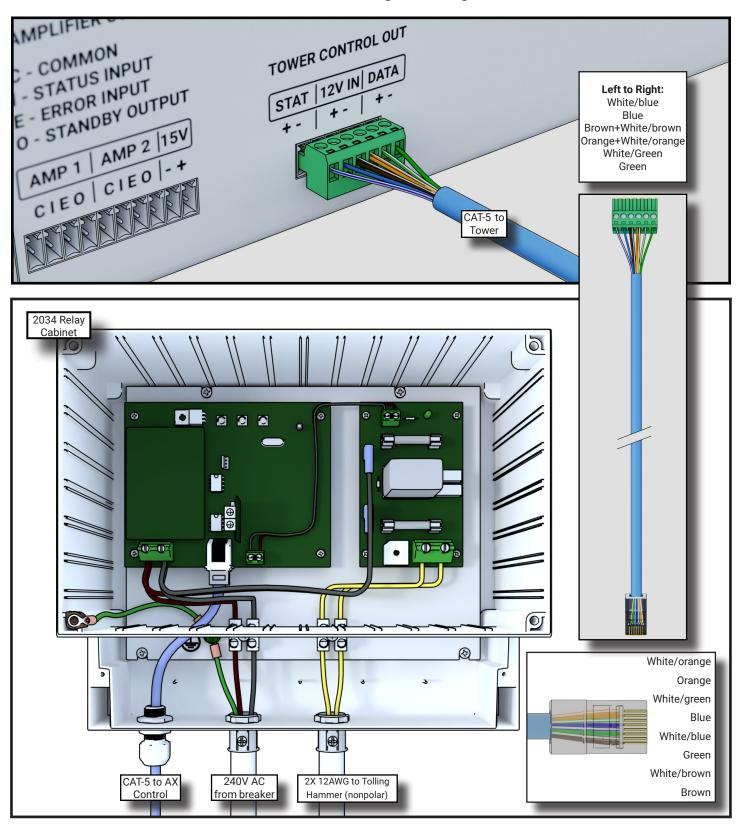
T1 configuration wiring schematic for one bell with Tolling Hammer. Chime Master shall furnish the AX controller, relay controller, and one tolling hammer with 32 inch pigtail (2 conductors + G).
